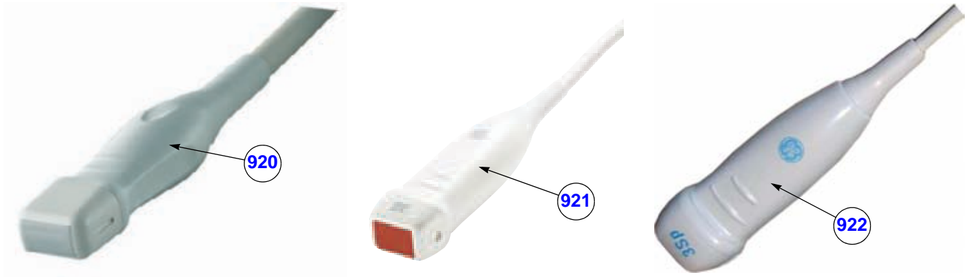
Figure 9-17 2D phased array Transducers
